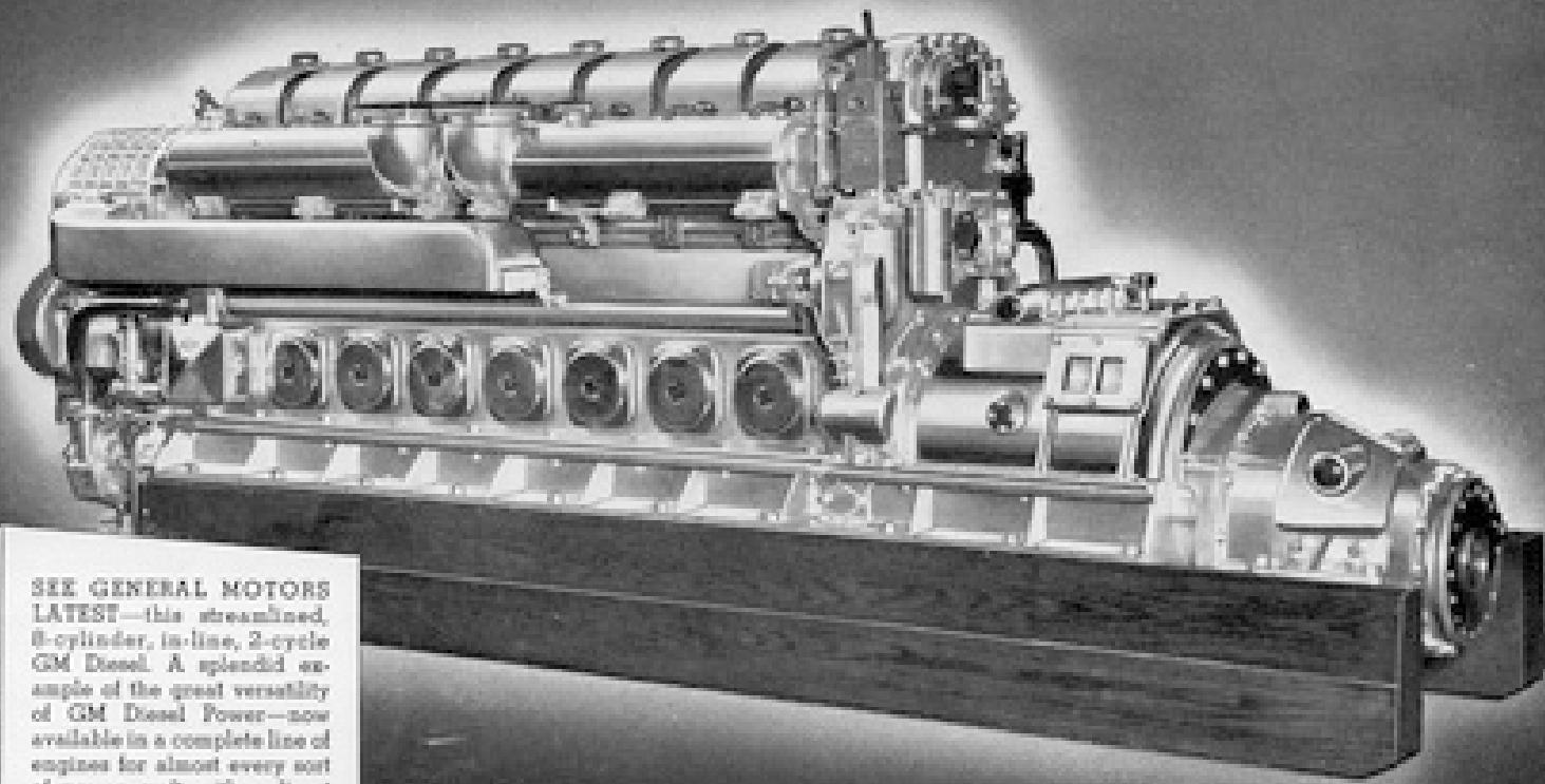
SEE GENERAL MOTORS LATEST—this streamlined, 8-cylinder, in-line, 2-cycle GM Diesel. A splendid example of the great versatility of GM Diesel Power—now available in a complete line of engines for almost every sort of power craft, either direct or electric drive.
